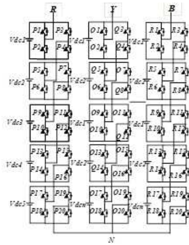
Fig. 8: 11-Level cascaded H-bridge inverter
